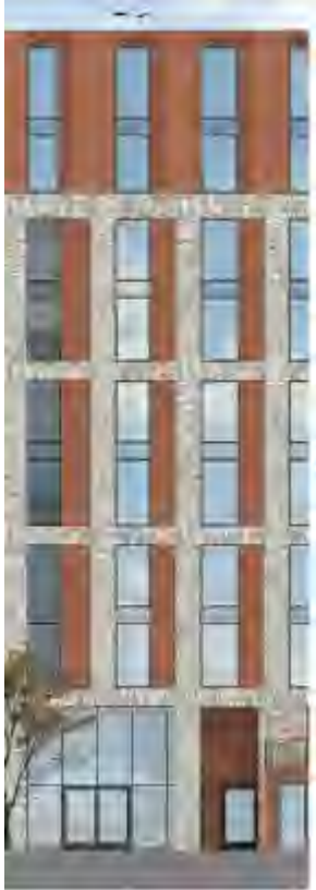
Typical bay study for buildings E and F with its masonry frame, inset panels, townhouse detail, double height entrance and Corten upper level
