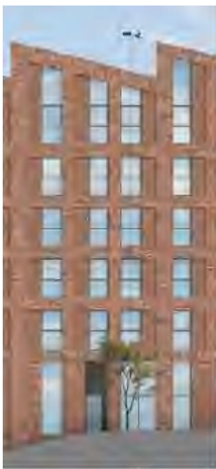
Typical bay study for building A with its sawtooth roof, decorative inset panel and masonry frame
